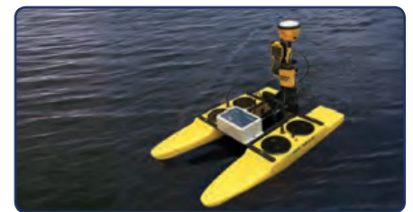
HyDrone™ ASV with Trimble SPS 585 and TSC3
