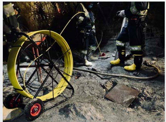
Carlson's Boretrak3 supports both surface and subsurface borehole deviation measurement
